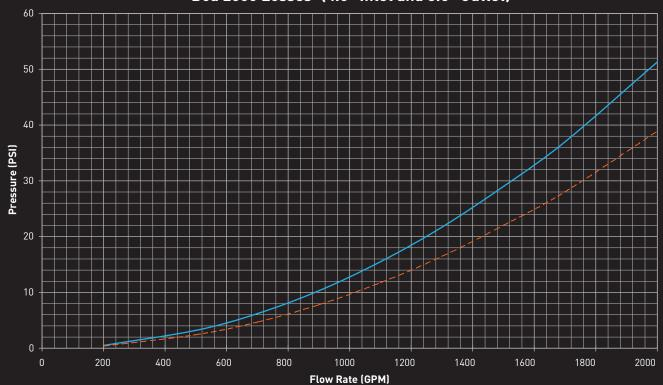
——Total Static Pressure Drop ——Friction Loss
